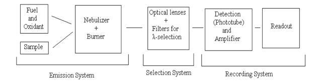
Figure 3. A general scheme of a Flame Photometer
