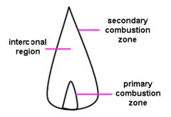
Figure 2. Schematic appearance of flame
