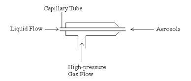
Figure 1. Design of a nebulizer
