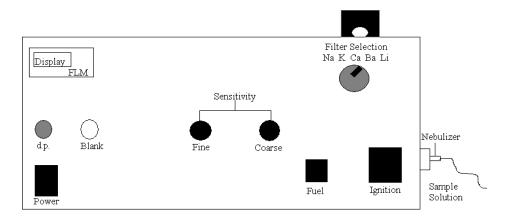
Figure 4. Front Panel Controls for the instrument
